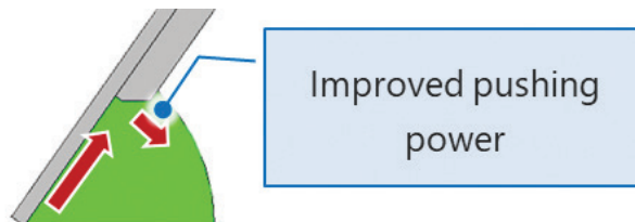
Figure 3. The 3SR squeegee improves aperture filling, paste rolling, and stencil lifetime.
